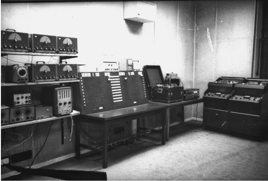
FIGURE 1.9 Electronic Music Laboratory at CLAEM, ca. 1964. Oscillators, noise generator, and filters are on the left; the original patchbay is at the center; Ampex recorders are on the right. Courtesy of Mary Mac Donagh de von Reichenbach.
