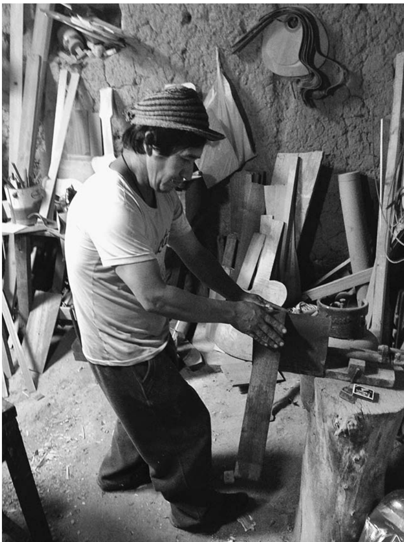
FIGURE 17. Marco bending chinlili sides over an open flame in his workshop. Photograph by author.
